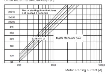
Rated current of fuse cartridge [A]
