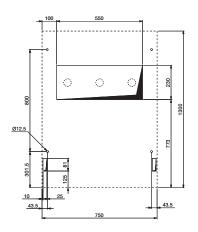
750 mm width for units with withdrawable circuit-breakers up to 24 kV WBS without cable outlet
