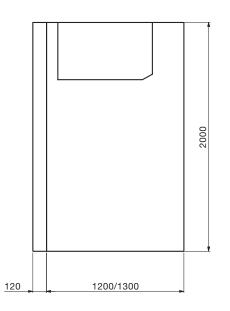
Side view for panels with withdrawable circuitbreaker, IAC A-FLR 25 kA, 1s up to 17.5 kV and IAC A-FLR 16 kA, 1s at 24 kV with filters
