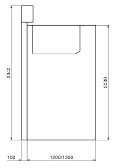
Side view for panels with withdrawable circuitbreaker, IAC A-FLR 25 kA, 1s up to 17.5 kV and IAC A-FLR 21 kA, 1s at 24 kV with duct
