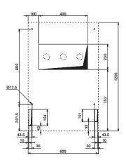
600 mm width for units with ithdrawable circuit-breakers up to 17.5 kV WBS and BME without cable outlet
