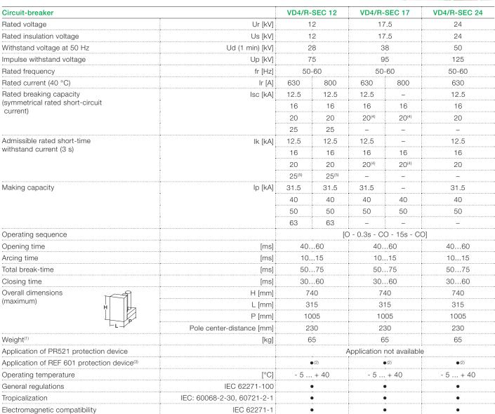
(1) Increase the indicated weight by 20 kg for circuit-breakers with REF 601 devices and 3 current sensors
